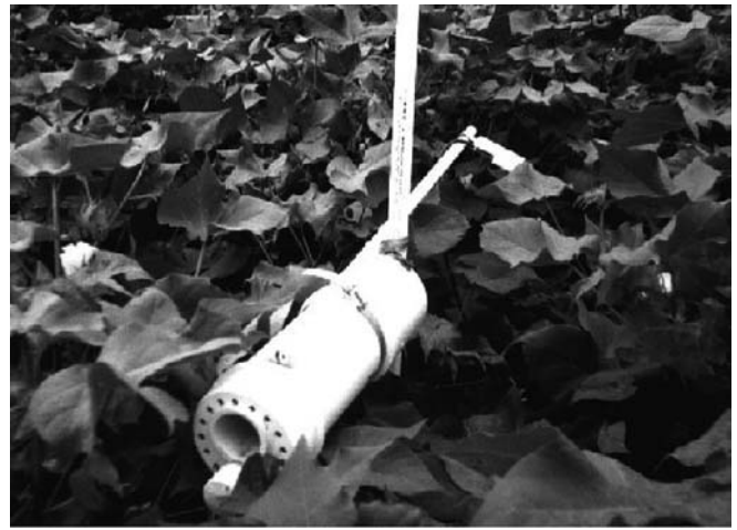
Fig. 1 Micro-station equipped with air temperature, relative humidity, and leaf wetness duration (LWD) sensors at the experimental cotton field
